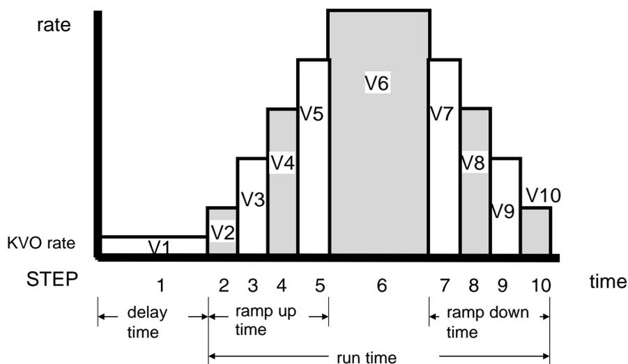
**Figure 5. Sample Ramp Program Delivery Profile (PDP)**
