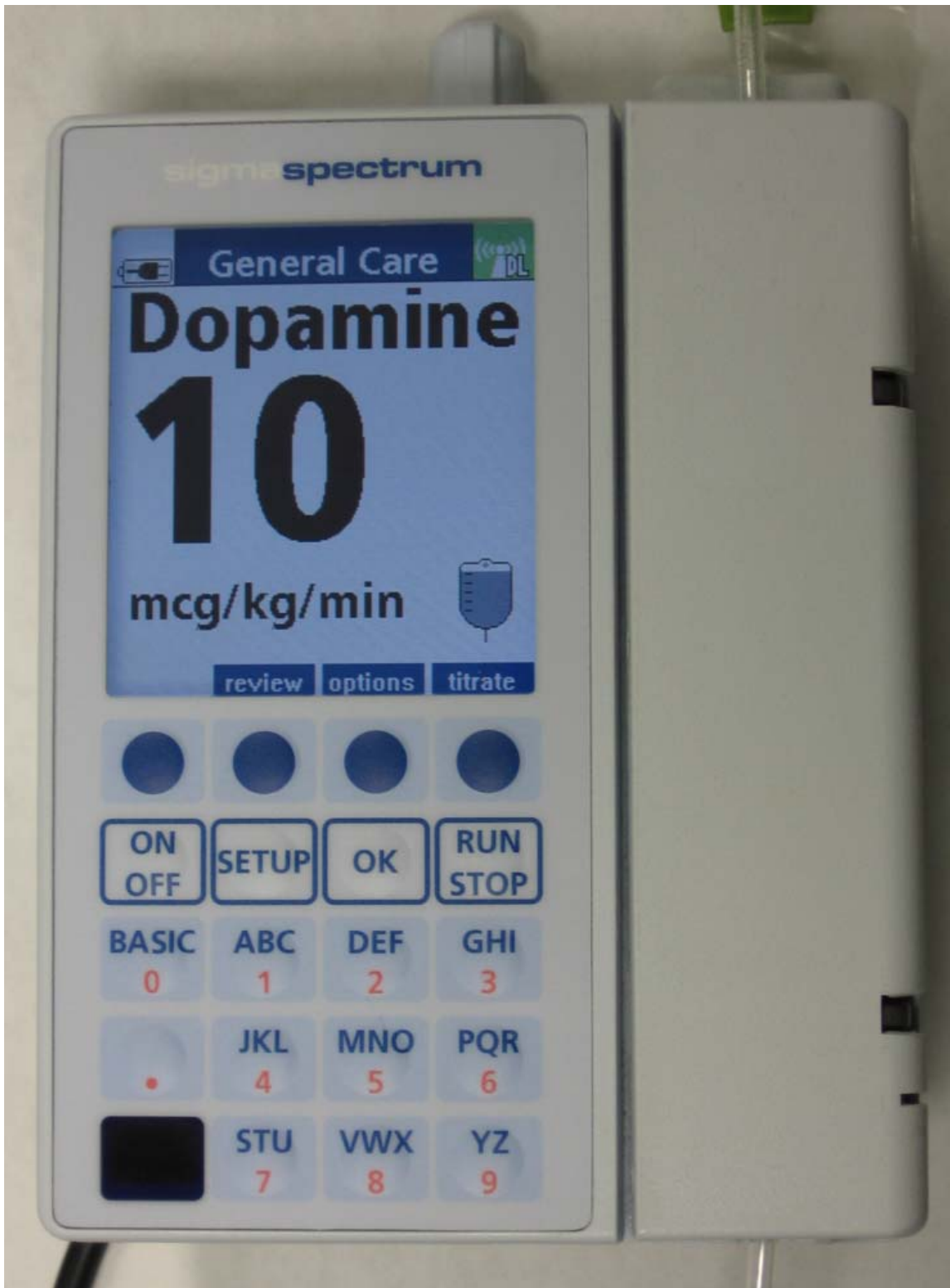
Front View – Pump Running with Wireless Battery Module
