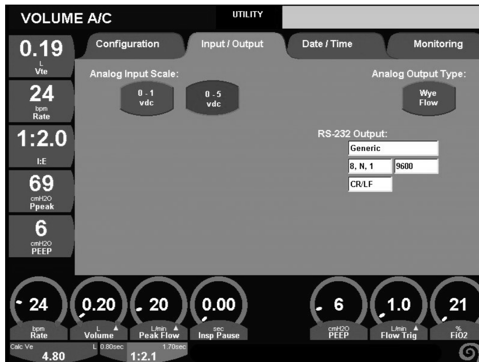
Figure 2–39: Utility Screen, Input / Output Tab, Generic RS-232 Output
