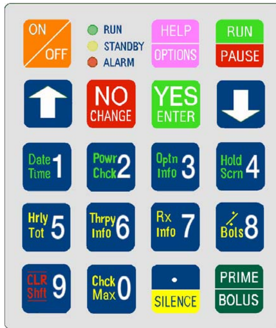
Figure 3.2. IOD Keypad with Info-On-Demand Feature
