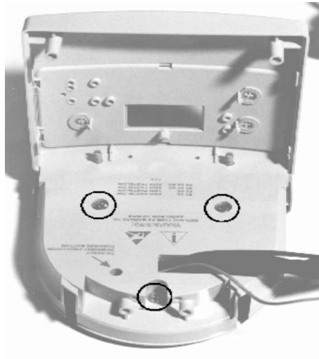
Figure 7.6 Showing location of Heater Plate screws
