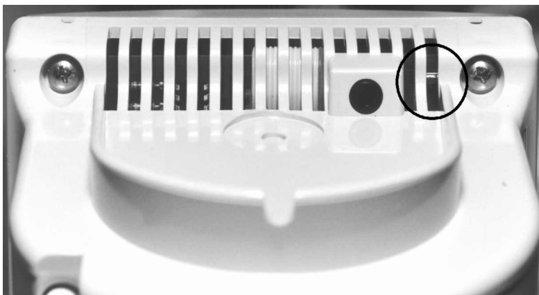
Figure 7.9 Showing Location of the Production Test Button
