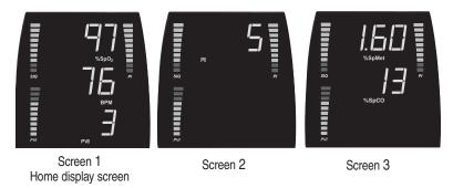
If SpMet and/or SpCO are not installed, the display will move from Screen 1 to Screen 2 when the Display Button is pressed; Screen 3 will not show. By pressing the Display Button again, the display will move from Screen 2 to Screen 1.
