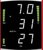
In addition to SpO2 and pulse rate, the Rad-87 allows you to select and display either SpHb, PVI or RRa on the main screen, with additional measurements displayed on subsequent screens accessed with the press of a button.
