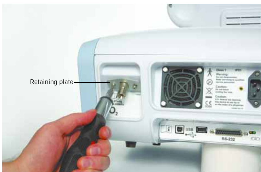
Figure A-3: Installing the oxygen inlet connector
