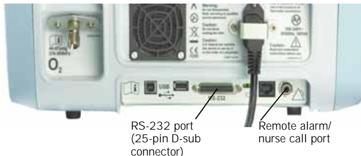
Figure B-1: Location of communications interface ports
