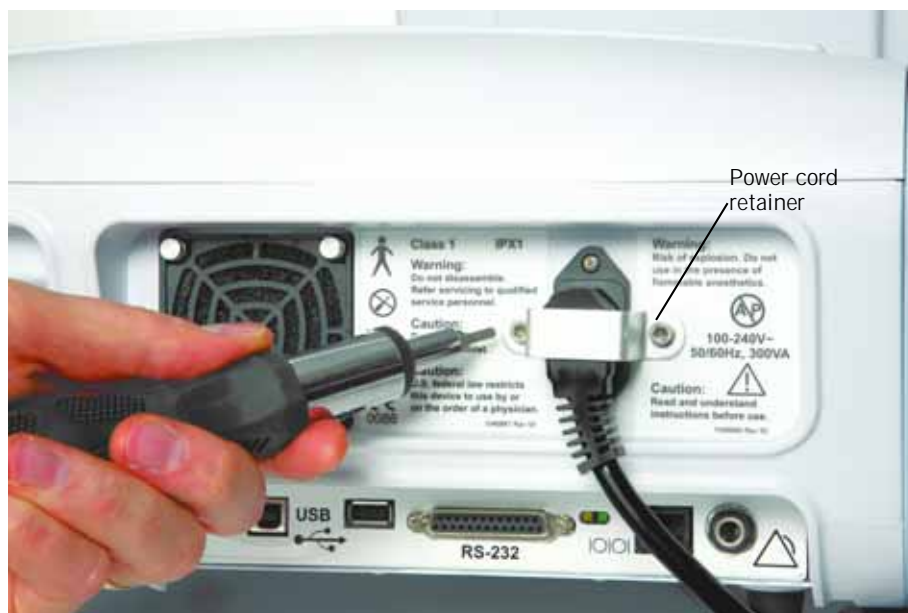
Figure A-4: Installing the power cord retainer
