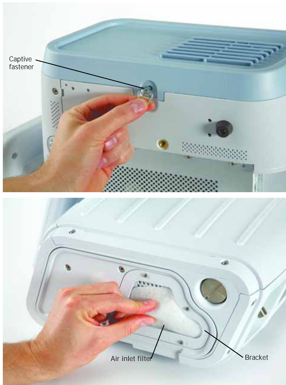
Figure 9-1: Replacing the air inlet filter
