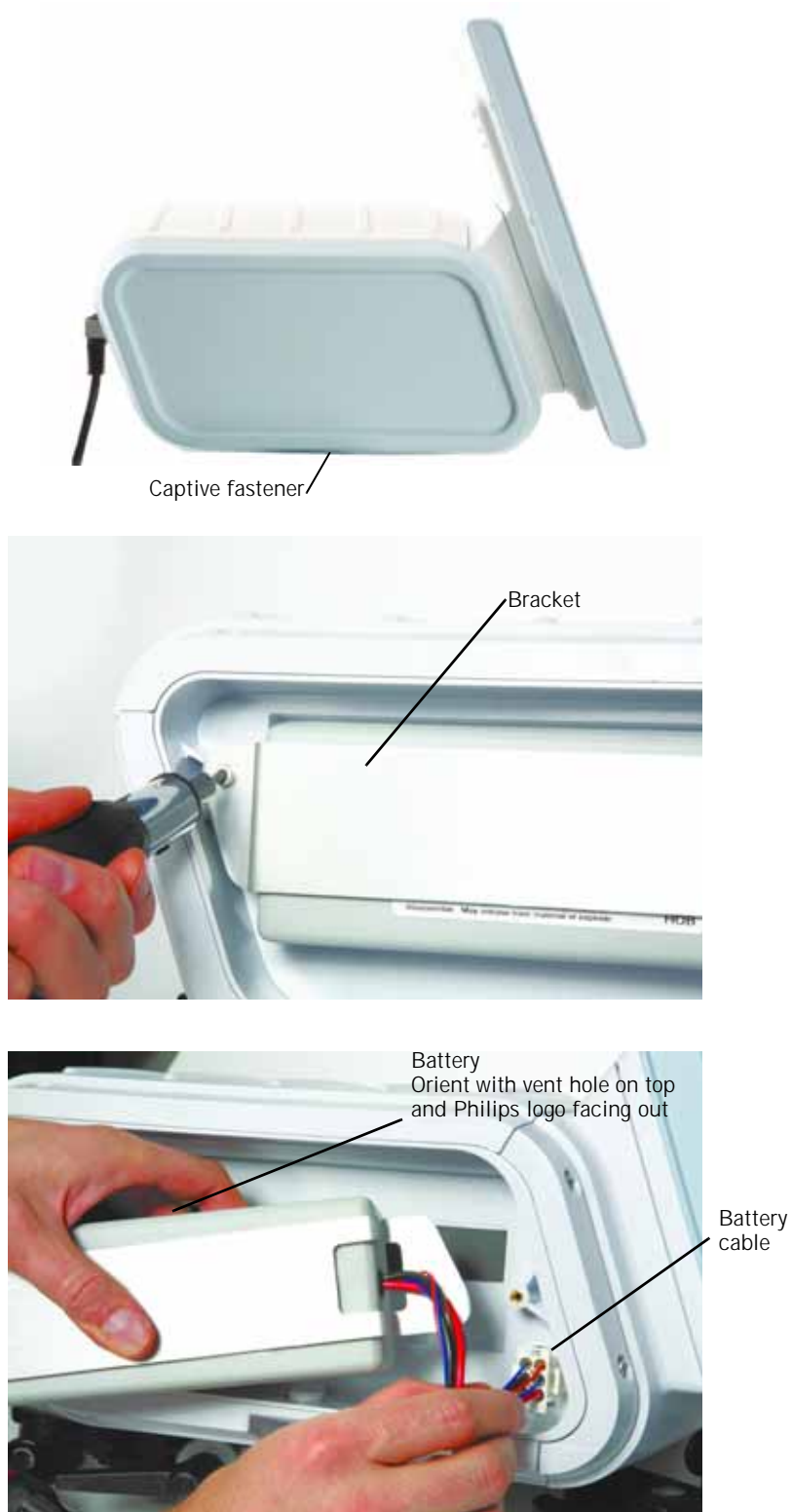
Figure A-2: Installing the battery
